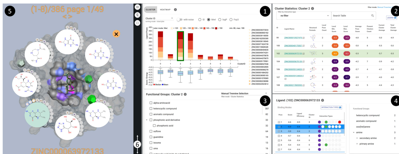
Fig. 1. InVADo Application Overview: ① Docking Overview : Visualizes the results of the clustered docking as a stacked bar chart combined with a box plot, where the bars represent the clusters. ② Statistics View : Gives cluster-specific information about ligands and their statistics in a tabular view with filter and sort options. ③ Functional Groups View : Provides cluster-specific information about functional groups (chemical substructures) of the ligands presented as an expandable and selectable treeview. It also extends the filter options of the Statistics View . ④ Ligand View : This table shows the individual binding poses offering ligand-specific details like the docking score and interactions. It is combined with a treeview presenting the functional groups of the current ligand. ⑤ 3D Visualization : Offers interactive visualization of the clustered docking results with a Radial Menu to browse them. ⑥ Sidebar Menu : Collapsible control panel allowing users to adjust the appearance of the 3D Visualization and to parametrize the clustering of the ligand binding poses and the functional groups.
